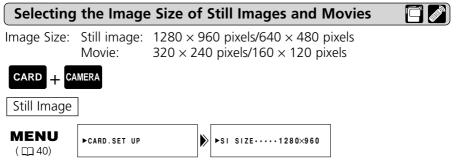
To change the image size of a still image, open the menu and select CARD SET UP. Then select SI SIZE, set it to "640  $\times$  480" and close the menu.
